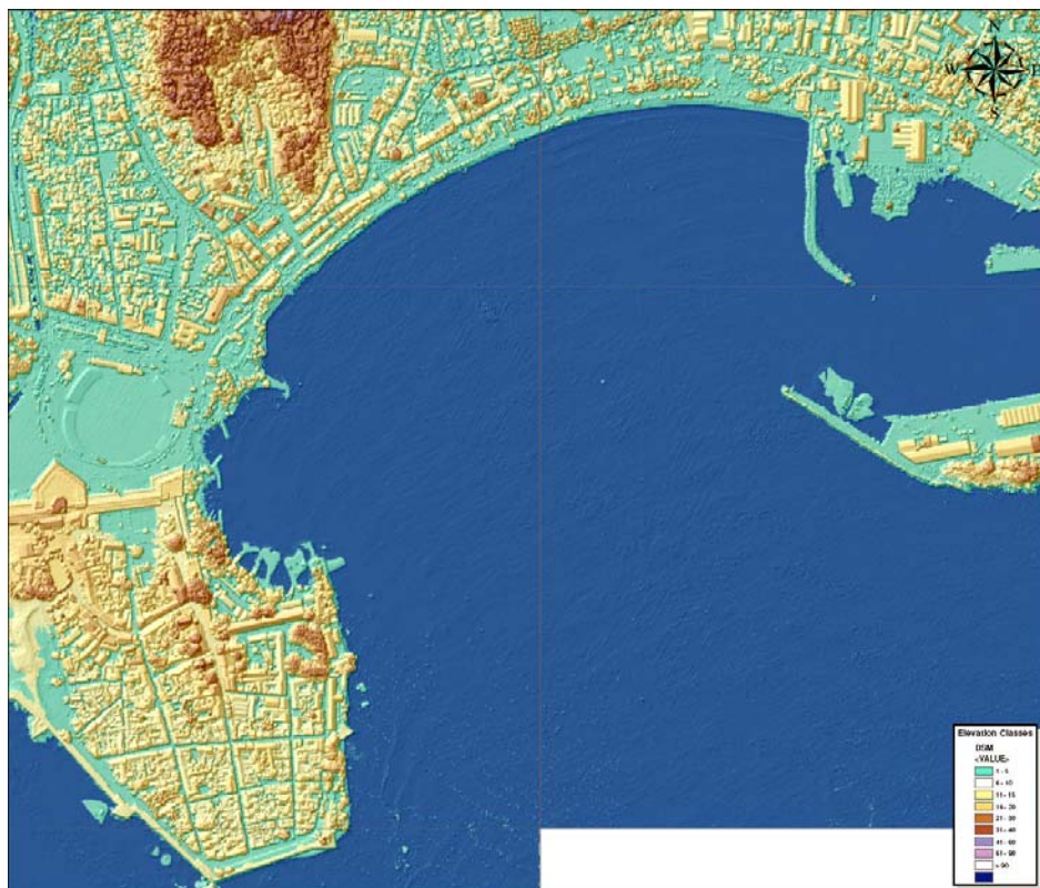
Figure 4. Shaded relief, LiDAR derived DSM of the seafront (centre), the harbour (right) and the 17 th Century Dutch fort (left) in the southern city of Galle. DSMs, obtained by mapping first returns from terrain - including buildings and vegetation - are better suited than DGMs to HyperDEM-like applications.
