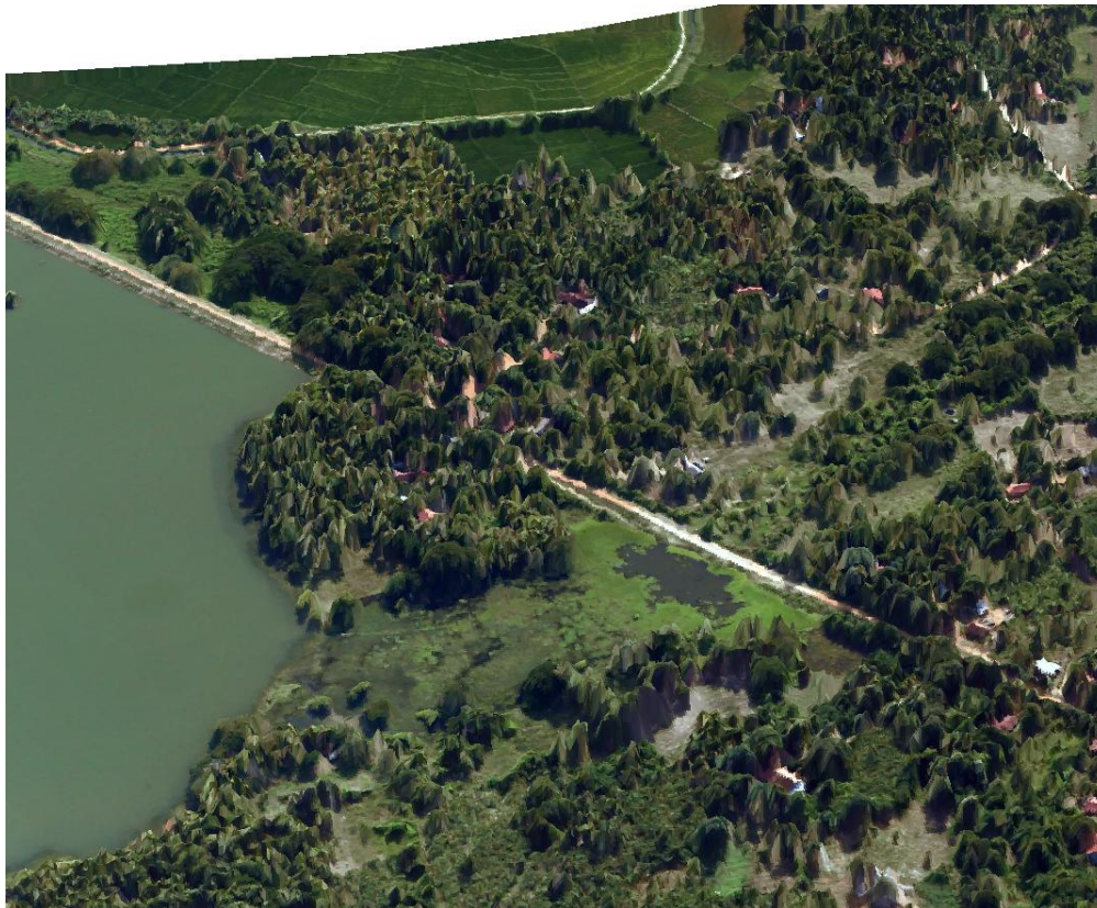
Figure 3. Example of 3D rendering of combined LiDAR (1m planimetric resolution, 0.2 m precision in elevation on steady reflectors) and digital camera aerial scenery (planimetric resolution of 0.2 m). This picture was taken over the artificial lake of Angunakolapelessa, southern Sri Lanka.
