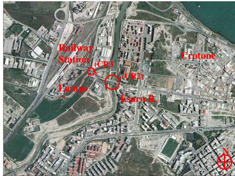
Figure 8. Critical sections considered for the critical urban area in Crotona: one on the Esaro River (CR2), corresponding to the road bridge along Nicoletta Street, the other (CR3) on the Lamps Creek before the flowing into the Esaro River.
