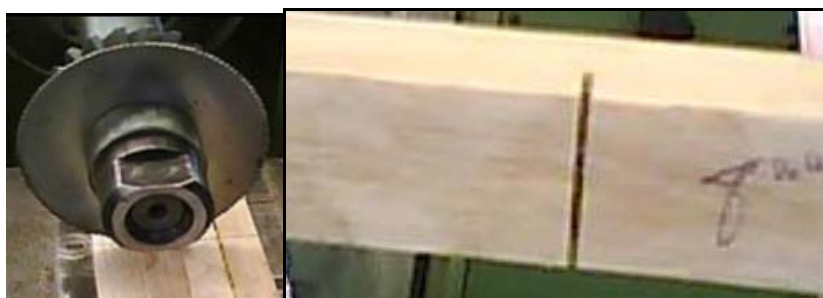
Figure 7. Specimens cut ( a_1 = 4\text{ mm} , a_2 = 8\text{ mm} )
