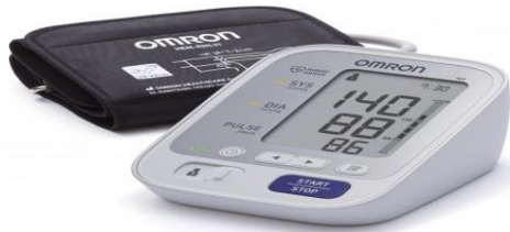
Figure 3. Electronic blood pressure monitor for measuring blood pressure and heart rate [14]
