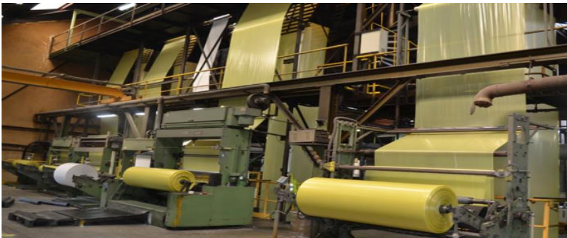
Figure I.8: Extrusion des films agricoles [16].
