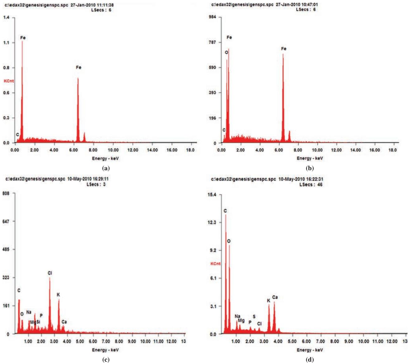
**Notes:** (a) Before immersion; (b) after seven days of immersion in 0.5M HCl without NE; (c) after seven days of immersion in 0.5M HCl with  $1.5 \times 10^{-3} \text{ g} \cdot \text{cm}^{-3}$  of NE; (d) of plant extract
