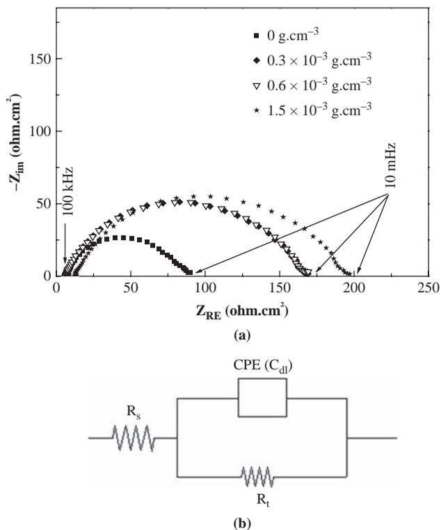
**Notes:**  $R_s$  – solution resistance,  $R_t$  – charge transfer resistance and CPE is the constant phase element of double layer capacitance  $C_{dl}$
