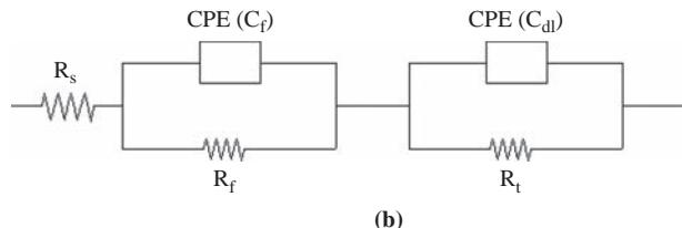
**Notes:** For example, and for clarity of the figure, is presented in the insert of (a), only the zoom of the HF loop for an immersion time of 8 h;  $R_s$  – solution resistance,  $R_t$  – charge transfer resistance and CPE is the constant phase element of double layer capacitance  $C_{dl}$ ;  $C_f$  and  $R_f$  are, respectively, the film capacitance and the film resistance caused by the adsorption of the inhibiting species
