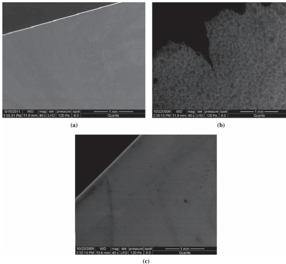
**Notes:** (a) Before immersion; (b) after seven days of immersion in 0.5M HCl without NE (border attacked by corrosion); (c) after seven days of immersion in 0.5M HCl with  $1.5 \times 10^{-3} \text{ g} \cdot \text{cm}^{-3}$  of NE
