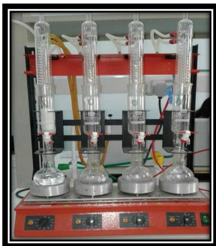
**Figure 14** : Appareil Soxhlet
