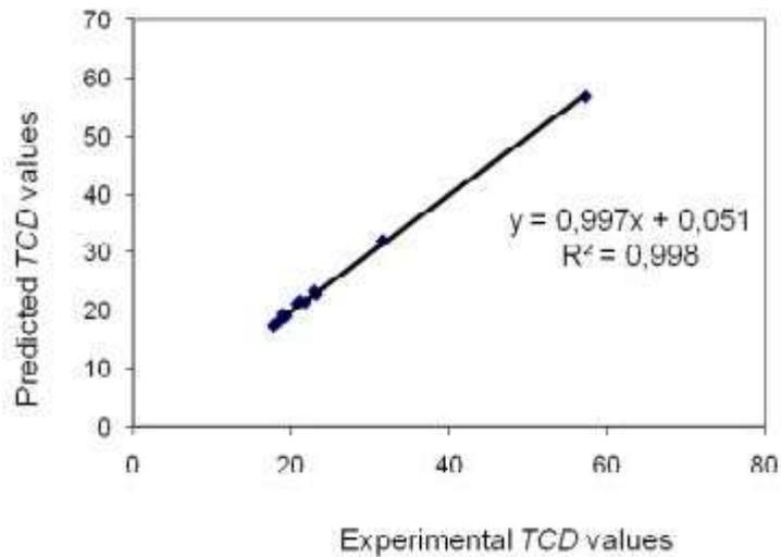
Fig. 3: Correlation between predicted and calculated TCD values. Case of MW-dried date pulp
