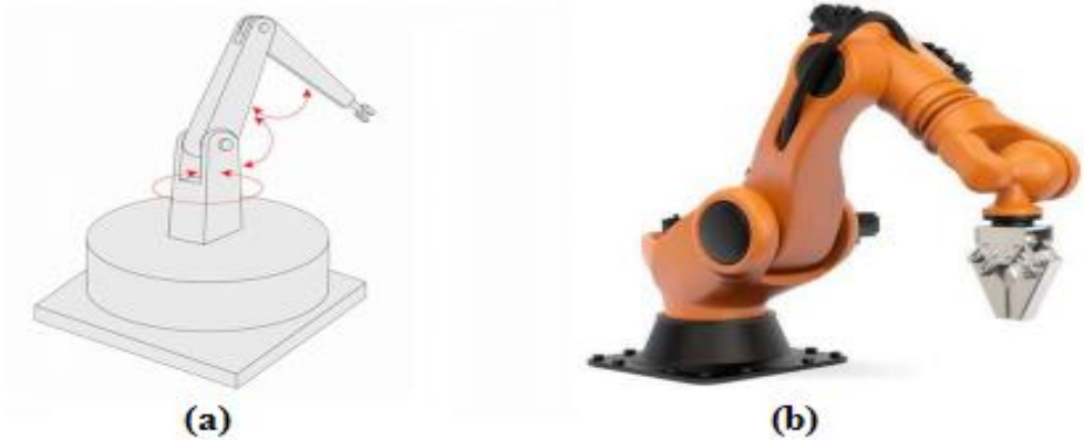
Figure I.15. (a) Structure anthropomorphic, (b) Robot anthropomorphic (Stäubli). [15]
