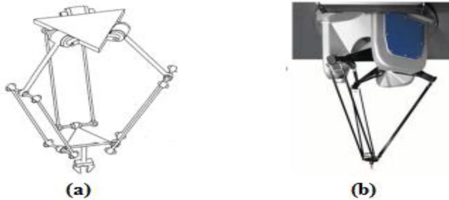
Figure I.6. (a) Structure parallèles DELTA, (b) Robot type DELTA. [15]
