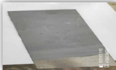
Figure III-2 : Application du " GALZINEPOX Gris ".
