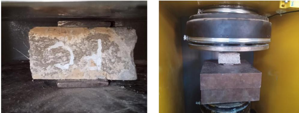
**Figure III. 21**: Essai de compression.
