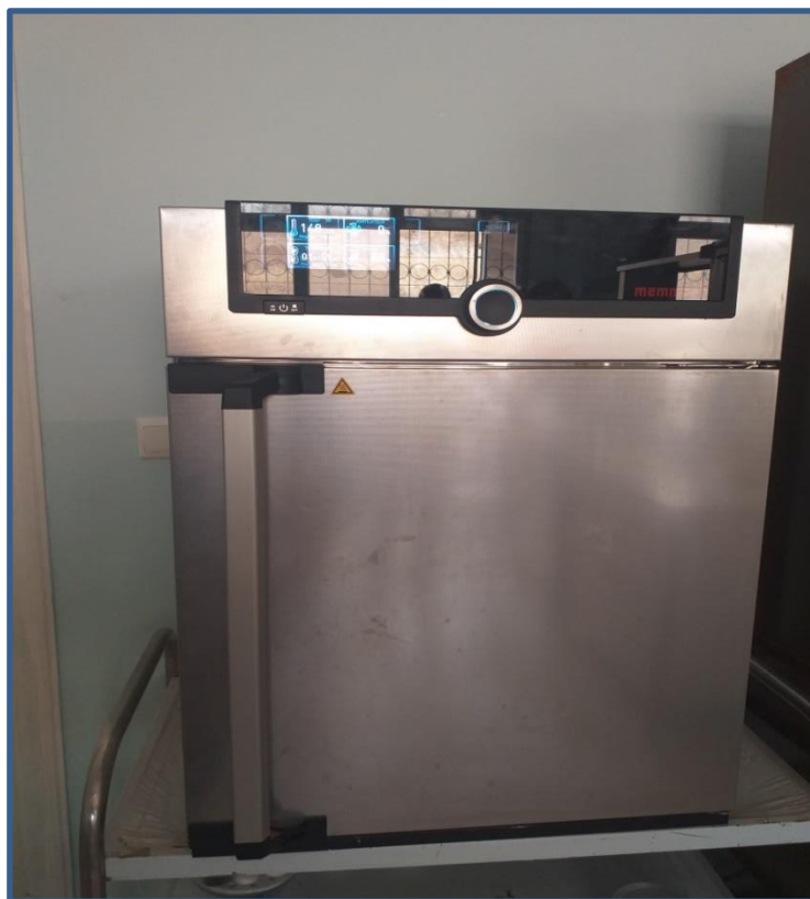
Figure II. 14: The furnace used to heat the substrate before deposition.
