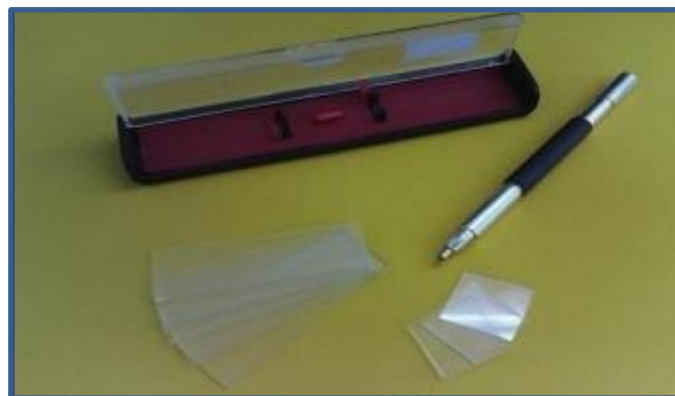
Figure II. 13: Cut glass substrate using diamond point pen.
