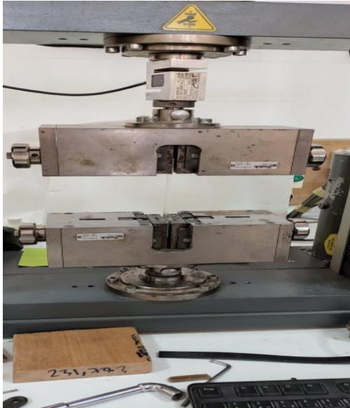
Figure IV. 8. La machine de traction Zwick /Roell/Z050
