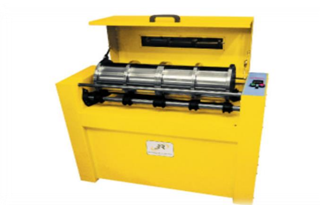
Figure III.3: Appareil Micro Deval
