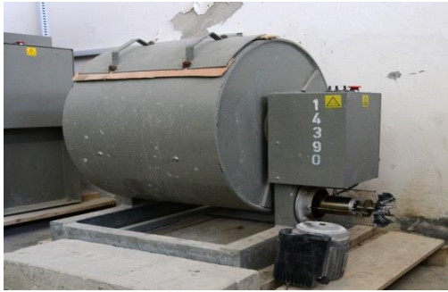
Figure III.4: Appareil Los Angeles
