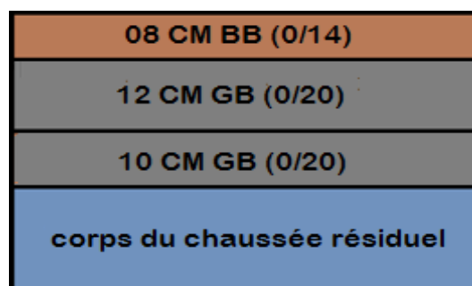
Figure IV.9 Illustration du renforcement de parking.
