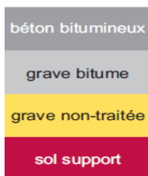
Figure I.3 structure chaussée souple
