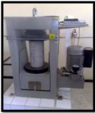
Figure.II.13 Presse de compression [20].
