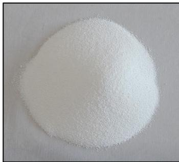
*Figure 0-6 Na<sub>2</sub>CO<sub>3</sub>*
