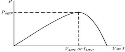
Figure 4: Power characteristic curve of GPV
