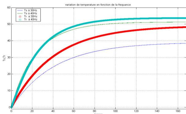
Fig. 8 stator and rotor temperature at 40 and 30 Hz
