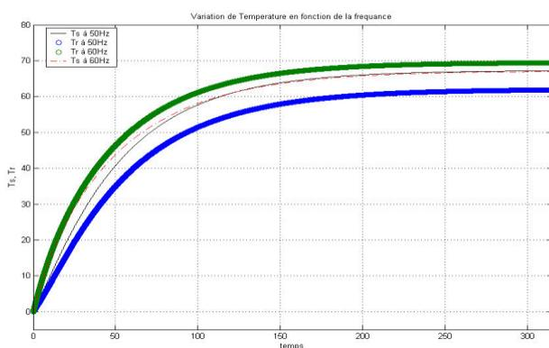
Fig. 9 stator and rotor temperature at -0 and 50 Hz
