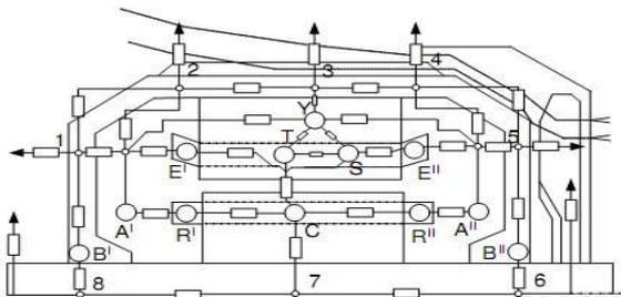
Fig. 5 Equivalent thermal models of the induction machine [4].
