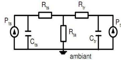
Fig. 6 Thermal model of the induction machine [7].
