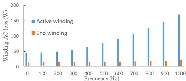
Fig. 1 Winding loss at different frequencies. Current amplitude:  $I_m=6A$  [21].
