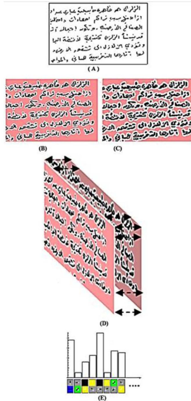
Figure 15. The steps of the oBIF column histogram (A) Original handwriting image (B) oBIF computation for scale parameter \sigma=8 and \sigma=4 (c) the oBIFs at two scales are crossed to form columns at each location (D) the histogram is computed with non-flat columns
