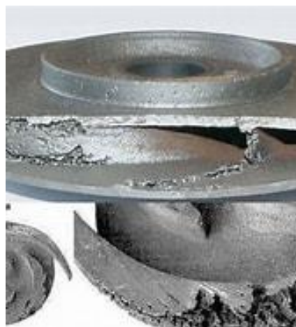
Figure 15: Effets de la cavitation (Arsizio, 2019)
