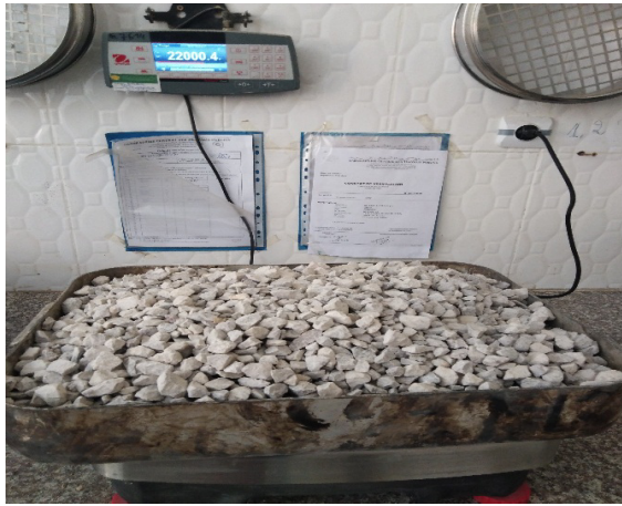
Figure [3.4] - Gravier 8/15 ( 22 \text{ kg/ m}^3 )
