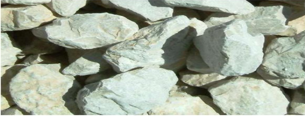
Figure I.3: grain de ballast de 30/60mm
