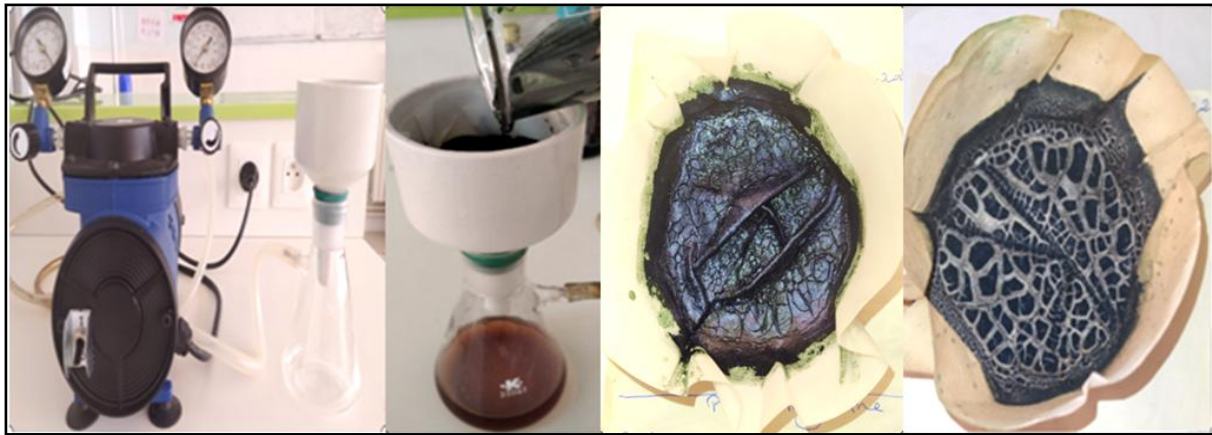
Figure II.03 : Protocole de filtration
