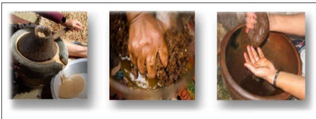
Figure 10: Trituration, malaxage et pressage manuel.
