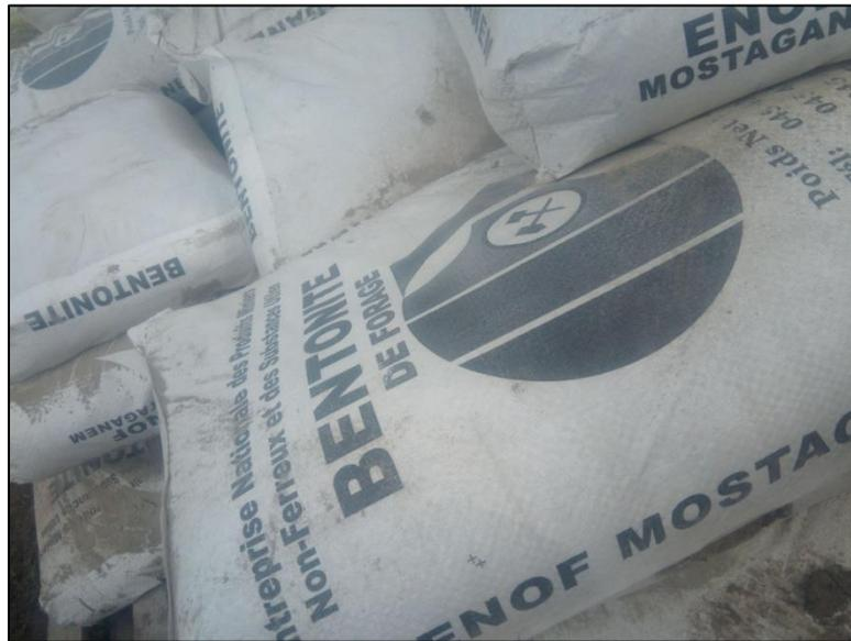
Figure 22: Bentonite de forage
