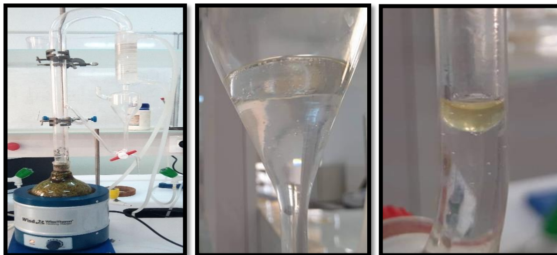
Figure III.4: Montage d'Hydro-distillation (Clevenger).
