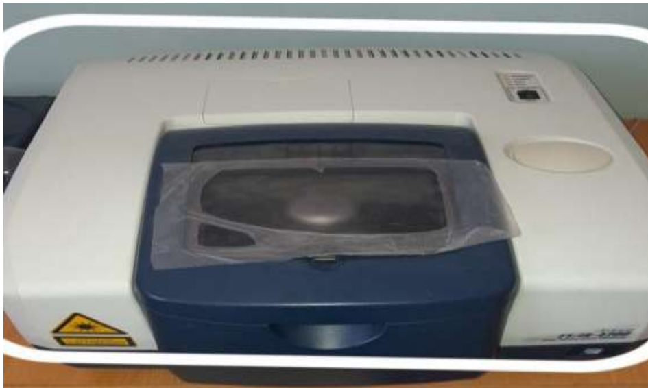
Figure II.5 : Appareil d'analyse IRTF Jasco 2400.
