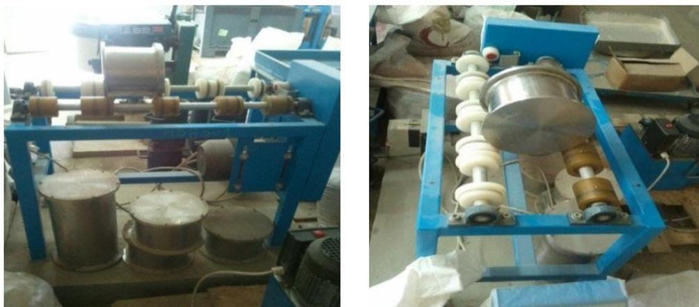
Figure I.10 : Machine D'essai Micro Deval [39].
