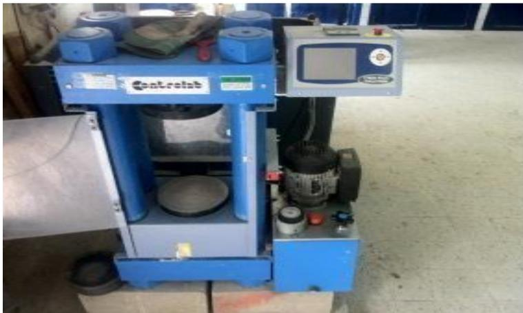
Figure IV.3: Machine d'essai de compression [83]
