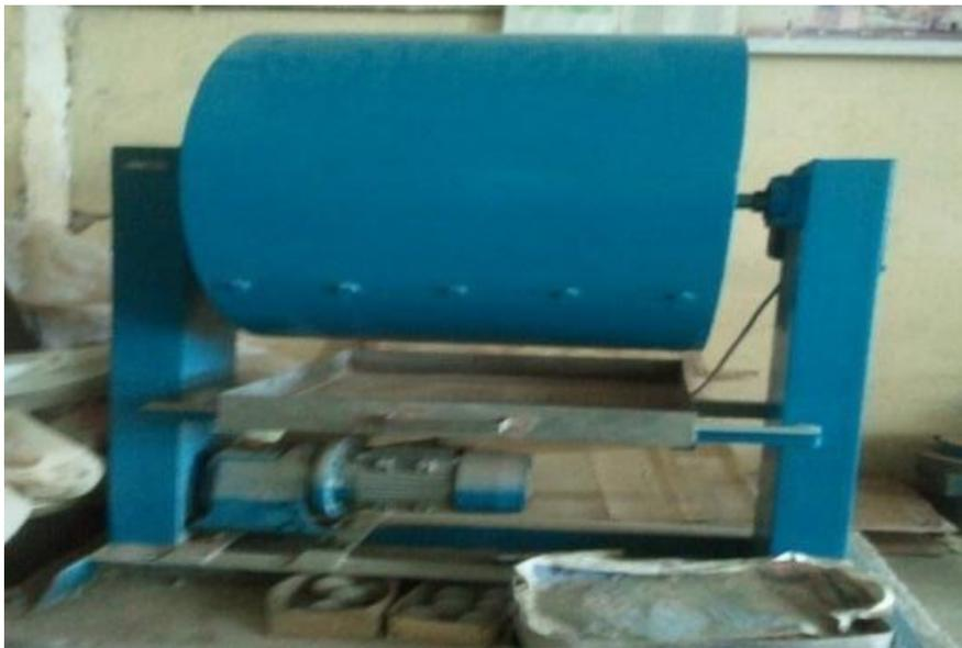
*Figure I.11 : Machine D'essai Los Angeles [41].*
