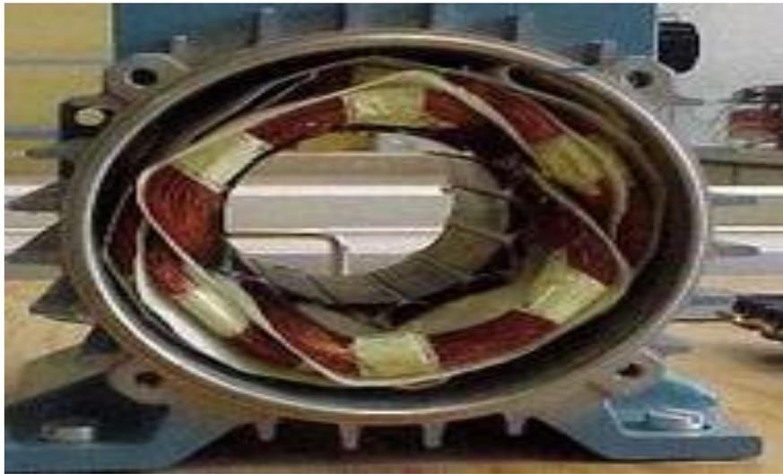
**Figure.I.1** : Stator.
