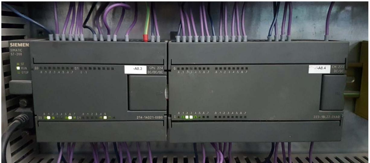
**Figure I.14** Automate SIEMENS S7-200.
