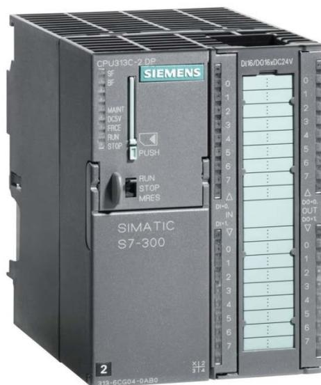
**Figure I.16** Automate SIEMENS SIMATIC S7-300.
