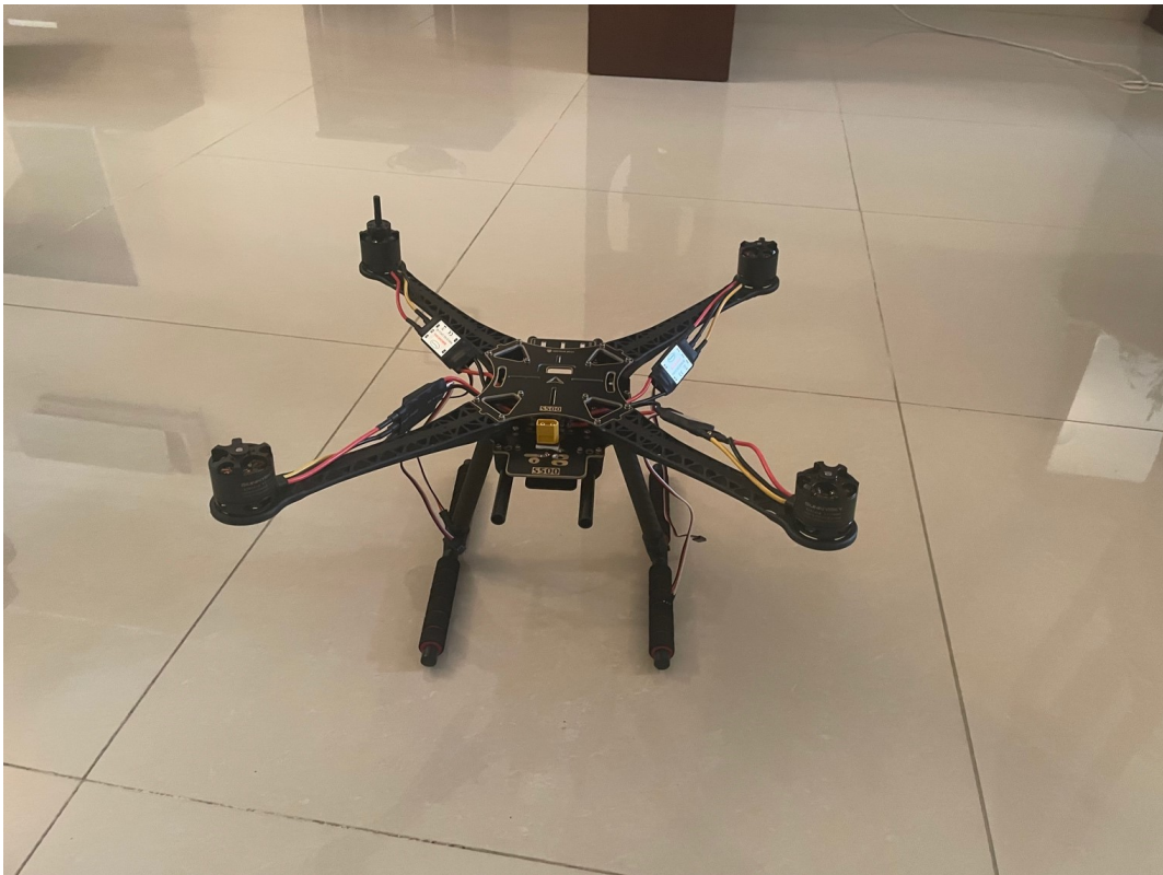
Figure 3.19 – frame assembly with motors, ESCs and PDB
