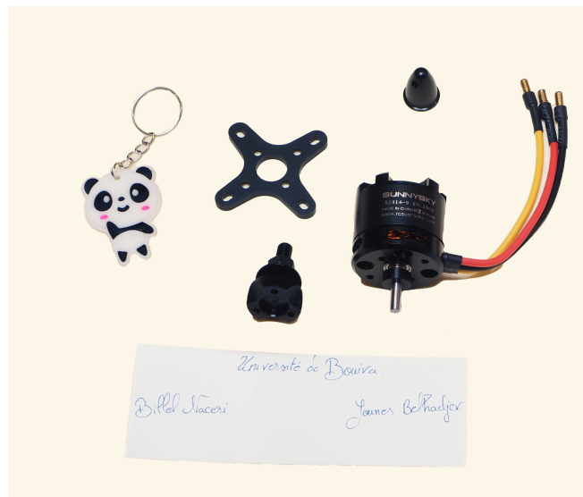
Figure 3.2 – Sunnysky 1000 KV “brush-less DC motor”
