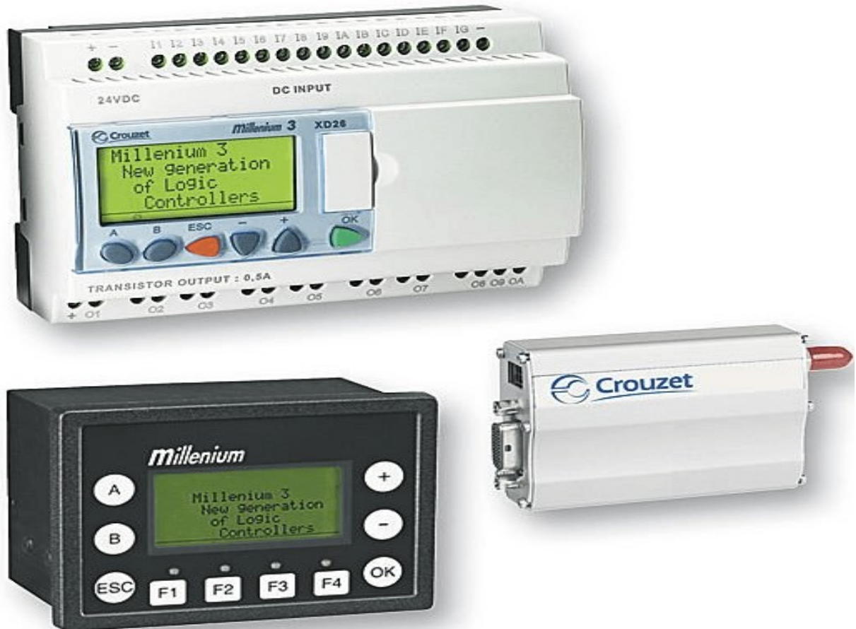
Figure I.14 : Programmable Logic Controller (PLC). [21]
