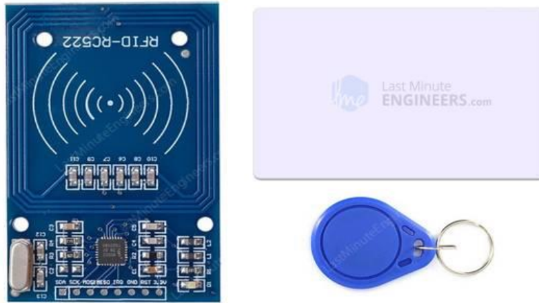
Figure (III.26) : module RFID [35].
