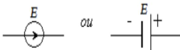
FIGURE 3.6 – Source de tension
