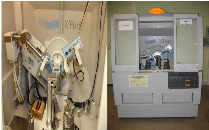
Figure II-5 : DRX de type PANALYTICAL XDR. X Pert PRO
