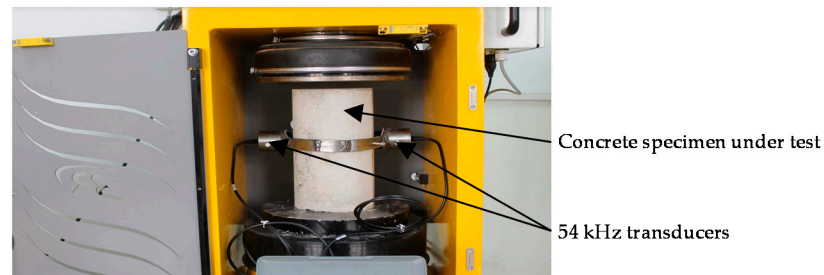
Figure 5. Ultrasonic NDT during compression of a concrete specimen.
