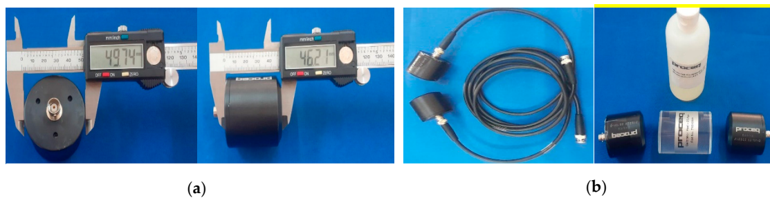
Figure 6. Some specifications on sensors and their use. (a) Transducer diameter and transducer length; (b) 2 transducers, 2 BNC cable and couplant + calibration rod.
