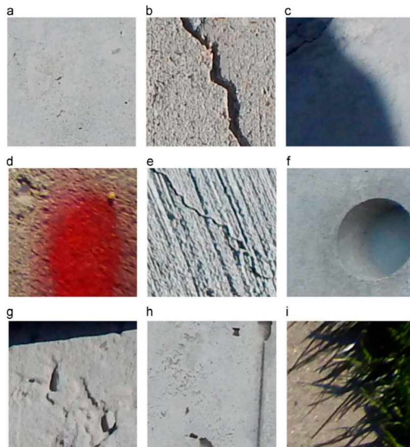
Figure 18. SDNET2018 (a) fine cracks, (b) coarse cracks, (c) shadows, (d) stains, (e) rough surface finishes, (f) inclusion sand voids, (g) edges, (h) joint sand surface scaling, and (i) obstructions.
