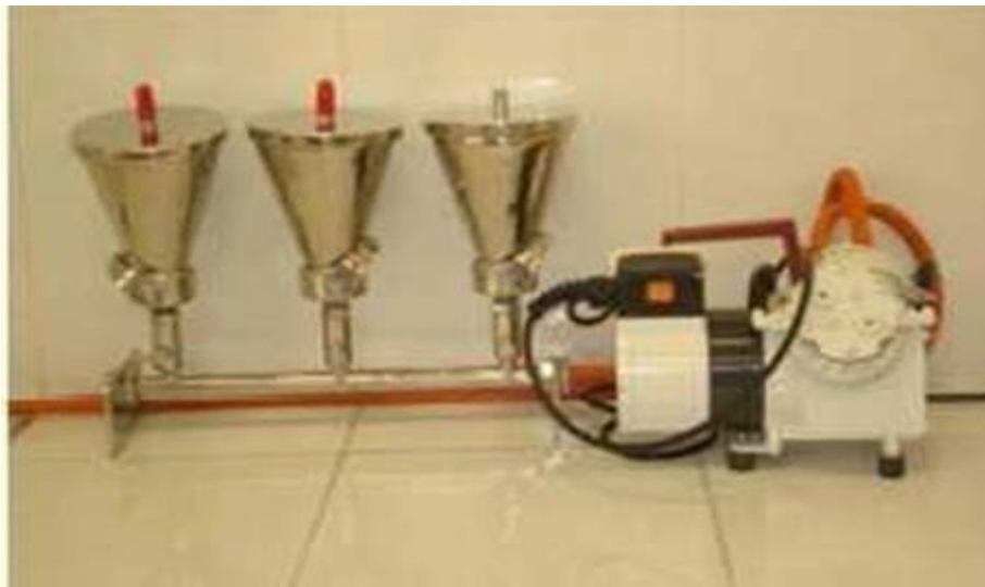
Figure II.3: filtration sous vide
