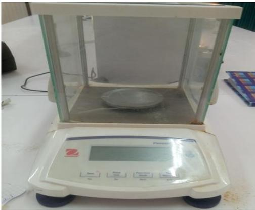
A photograph of an analytical balance, specifically an Ohaus model. It features a white base with a digital display and control buttons. A glass weighing chamber is mounted on top, and a weighing pan is visible inside. The device is placed on a white surface.                         |
