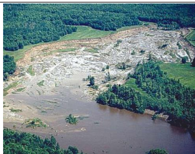
Figure I-18: The 1993 Lemieux landslide a rapid earth flow in sensitive marine clay near Ottawa, Canada. [1]
