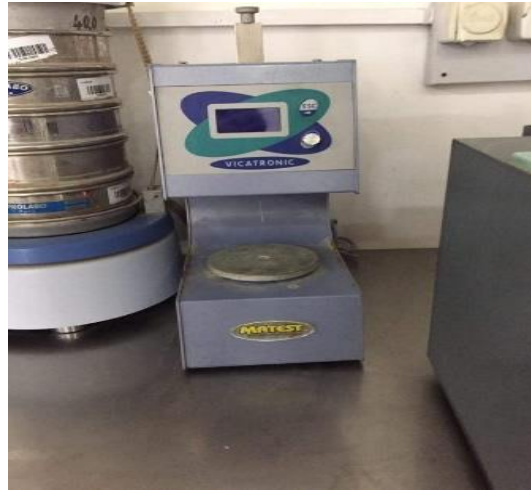
FIGURE II.1 : ESSAI DE PRISE VICATORNIC.
