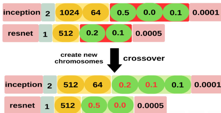
Figure 3.13: An example of the crossover phase using the TL encoding system.
