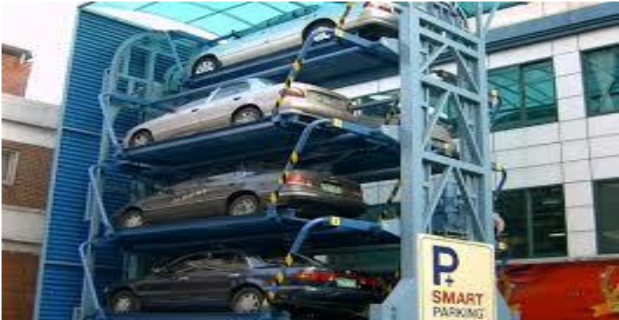
Figure I.7: Parking double l'emplacement vertical [2]
