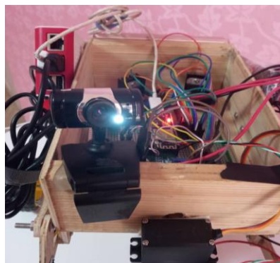
Figure 4. 14. Alimentation de la webcam.
