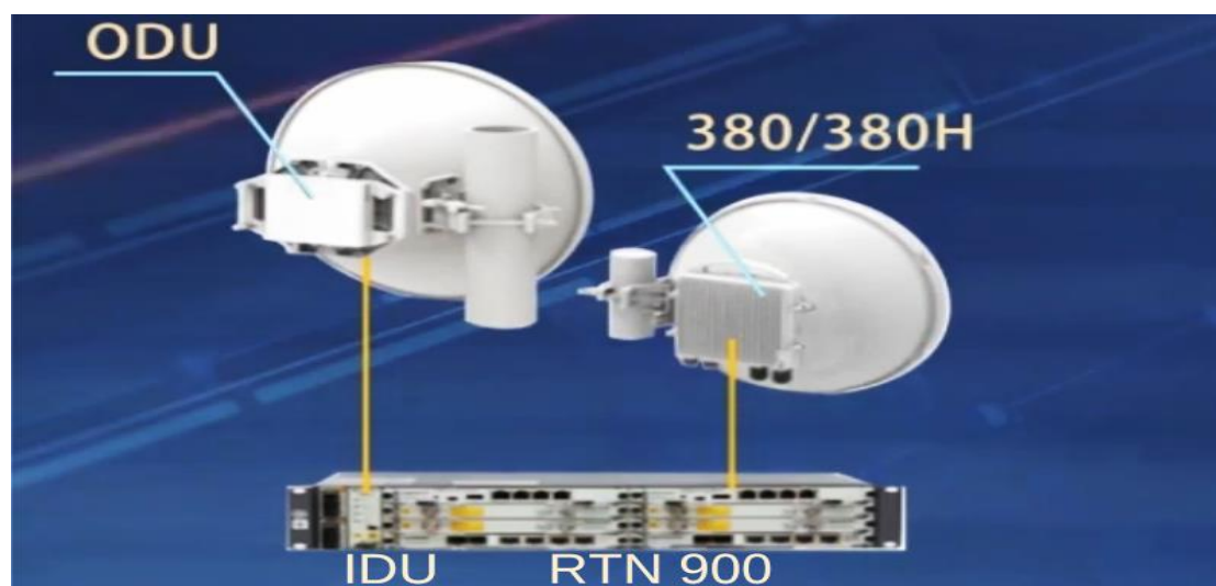
Figure III. 4: L'architecture de la solution Super Dual Band.
