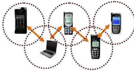
Figure 1.3: Mobile Ad hoc Network
