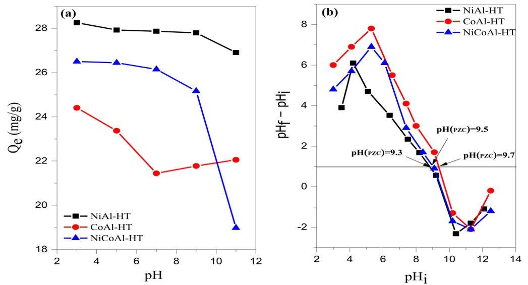
**Figure 7.** Effect of initial solution pH on TY uptake ( $C_0 = 100 \text{ mg}\cdot\text{L}^{-1}$ ,  $m = 80 \text{ mg}$ ,  $V = 20 \text{ mL}$ ,  $T = 25 \text{ }^\circ\text{C}$ ) (a), Zero point charge determination (b).
