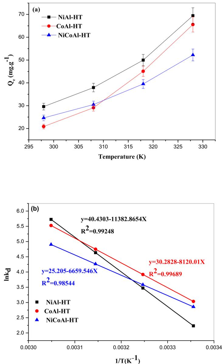
**Figure 11.** (a) Impact of temperature on TY uptake onto NiAl-HT, CoAl-HT, and NiCoAl-HT ( $C_0 = 100 \text{ mg}\cdot\text{L}^{-1}$ ,  $m = 80 \text{ mg}$ ,  $V = 20 \text{ mL}$ ,  $\text{pH } 3$ ); (b) Evolution of  $\ln K_d$  as function of  $1/T$ .
