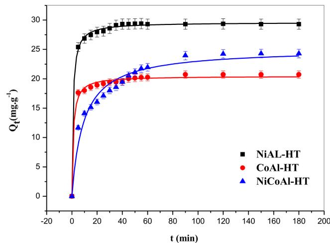
**Figure 9.** Non-Linear regression plots of Pseudo-second-order kinetic model for the adsorption of TY onto NiAl-HT, CoAl-HT, and NiCoAl-HT ( $C_i = 100 \text{ mg}\cdot\text{L}^{-1}$ ,  $\text{pH} = 3$ ,  $D = 4 \text{ g}\cdot\text{L}^{-1}$ ,  $T = 25 \text{ }^\circ\text{C}$ ).
