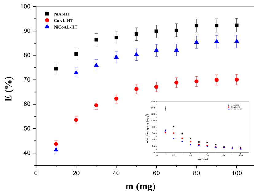
**Figure 8.** Removal efficiency of TY as a function of the mass of adsorbents NiAl-HT, CoAL-HT, and NiCoAl-HT and the adsorption capacity ( $C_i = 100 \text{ mg}\cdot\text{L}^{-1}$ ,  $V = 20 \text{ mL}$ ,  $T = 25 \text{ }^\circ\text{C}$ ).
