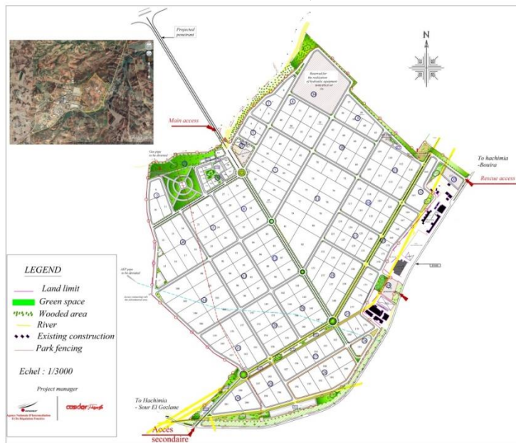
Figure 8: Parcel plan of the Oued El Berdi industrial park (Sidi Khaled Extension)
