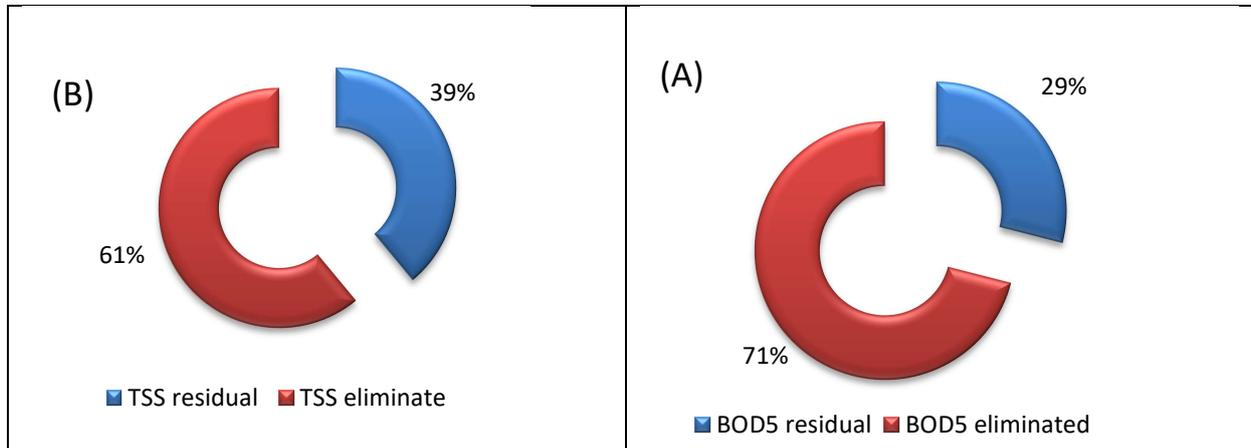
**Fig 13.** BOD<sub>5</sub> removal rate (A), TSS removal rate (B)
