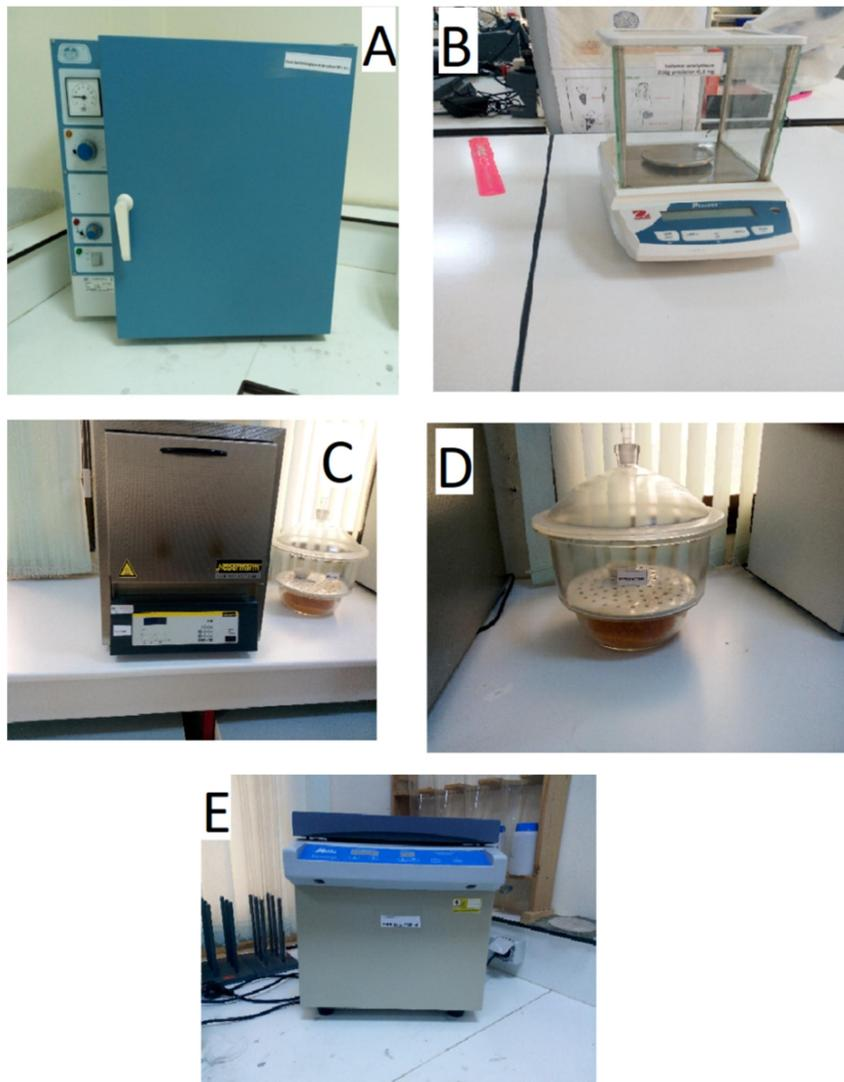
**Fig 7.** Oven (A); Scale (B); Furnace (C); Dryer (D); Centrifuge (E)
