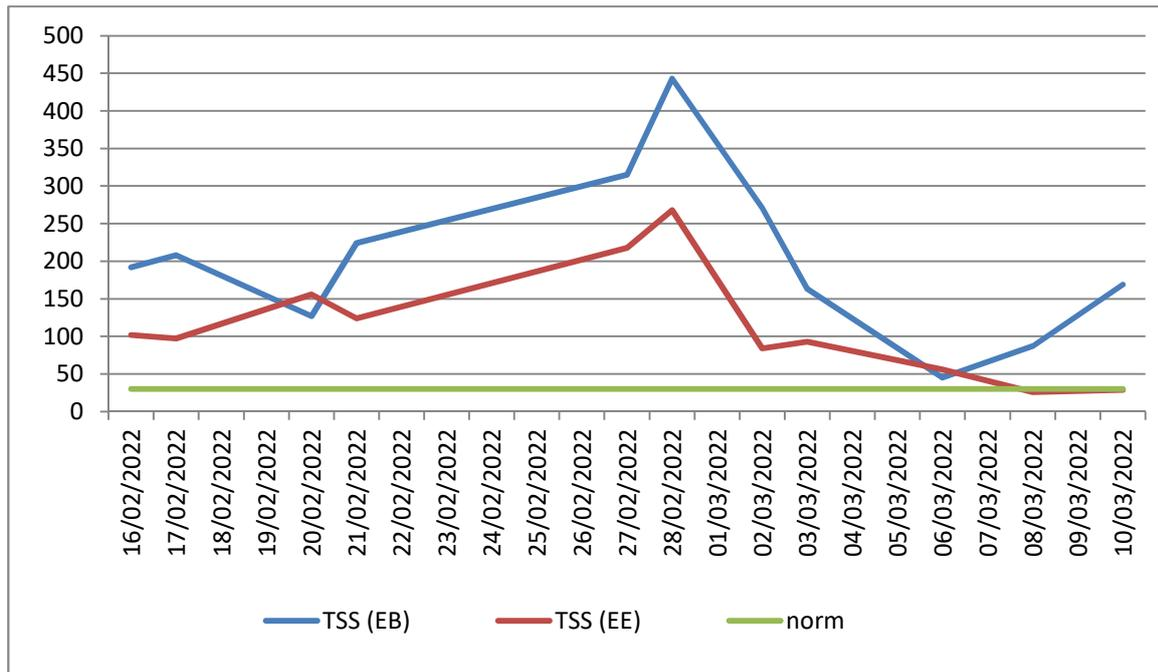
**Fig 11. Variation of TSS of raw water and purified water**
