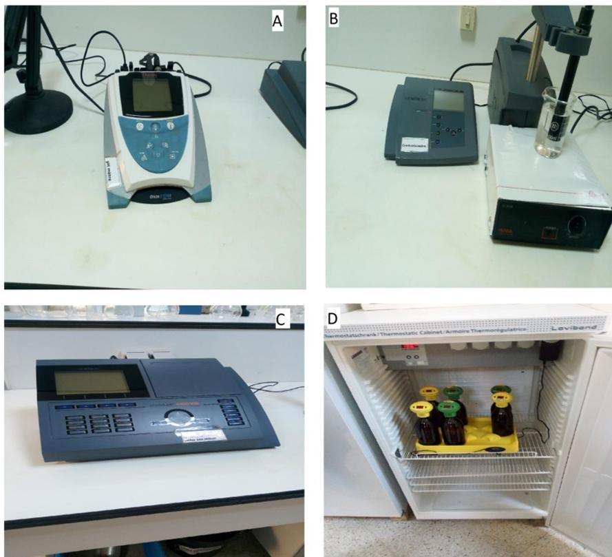
**Fig 5.** PH meter (A); Conductivity meter (B); Spectrophotometer (C); Incubator (D)
