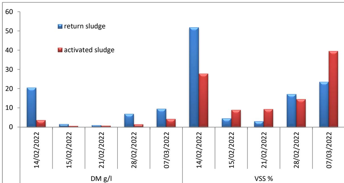
**Fig 14.** Variation of DM and VSS of Returned Sludge and Activated Sludge
