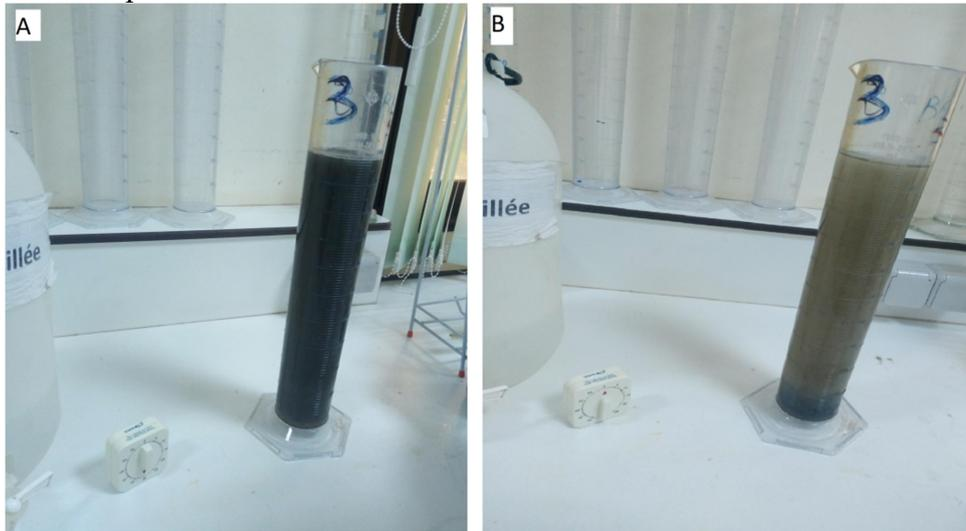
**Fig 6.**  $V_{30}$  before decantation (A), decantation after 30min (B)
