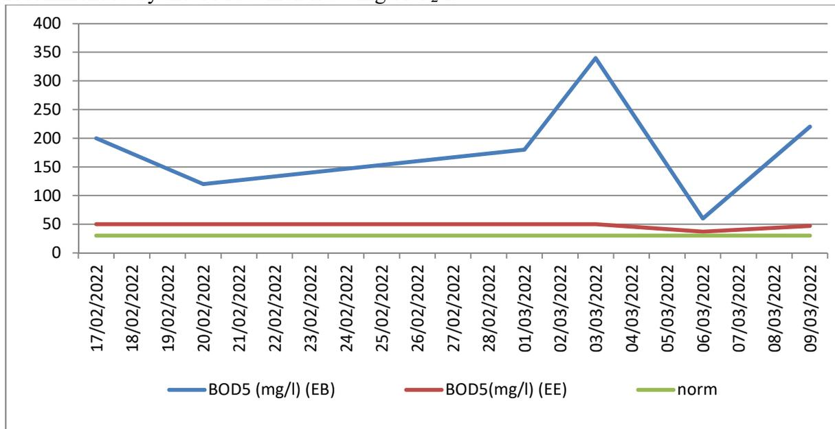
**Fig 12. Variation of BOD<sub>5</sub> of raw water and purified water**
