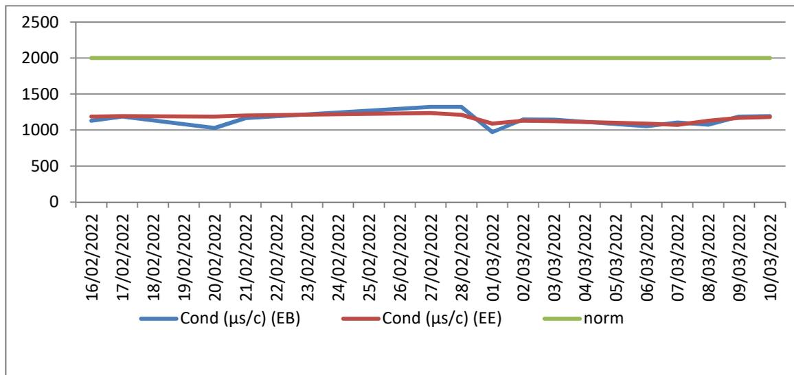
**Fig 09. The conductivity of the raw water and the purified water.**
