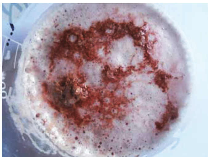
Fig. 10. Picture of agglomerates formed in the aphron phase recovered from the separation trials carried out with undiluted extract [46]
