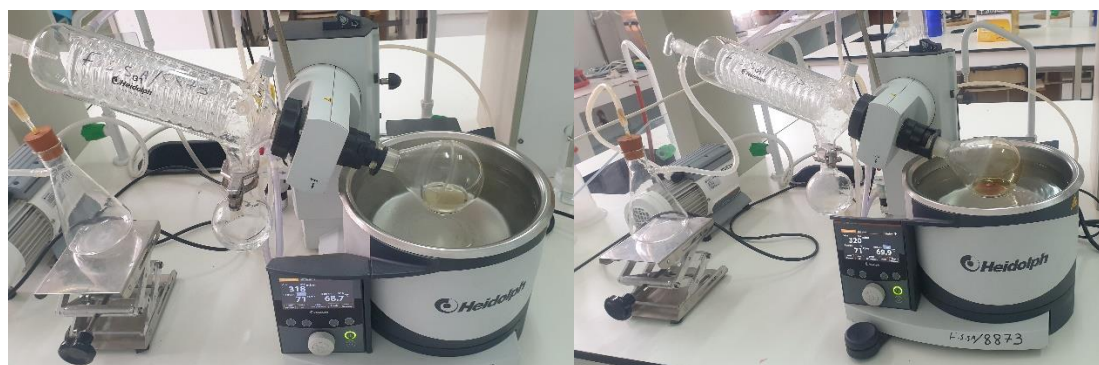
Figure 24. Evaporation of extracts (fruits and seeds) using a rotary evaporator. (Original, 2024)
